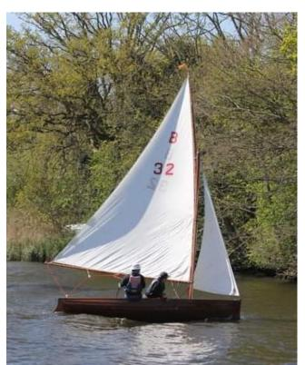
Built in 1935 of wooden mahogany clinker construction. Good usable condition and ready to sail straightaway.
